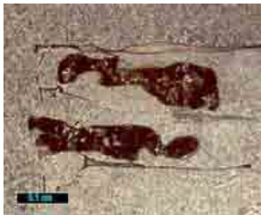
troilite, FeS, brown cohenite. (Fe,Ni) 3 C, white in taenite and kamacite matrix
